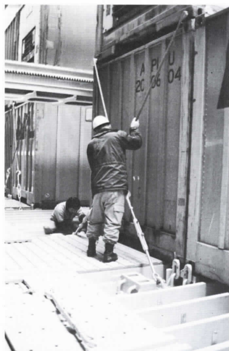
Lashing a second tier of containers on Spring Bird 's D deck.
