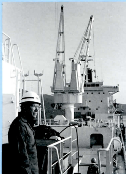
The cranes have been mounted high so as to provide room for operations with containers stacked in to layers. Lennart Lindau, technical manager of SRS, to the left.
