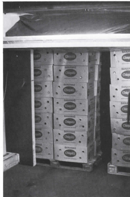
One of the Banana Company's ripening rooms which uses the new ripening method involving palletized bananas.
