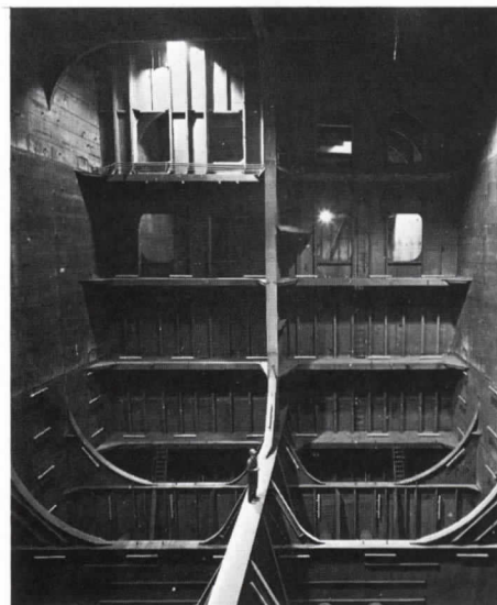
The center tank in one of Salén's tankers complying with the MARPOL Convention. It is equipped, among other items, with a Gunclean tank cleaning system.
