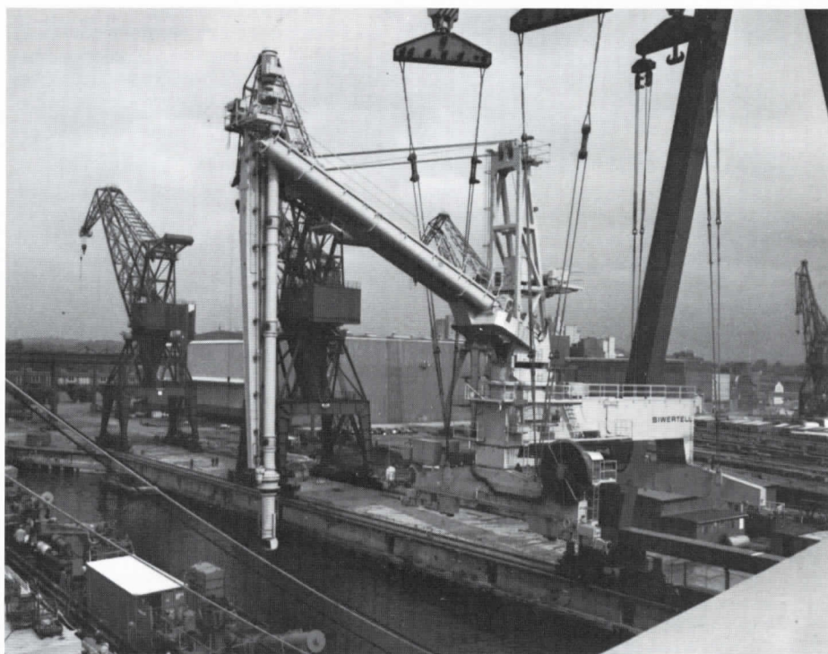
A Siwertell cement unloader is hoisted aboard a converted bulk carrier at the Eriksberg Shipyard in Gothenburg. Of the total of about 20 ships which were fitted with Siwertell equipment, the "Abu Mariam" and "Abu Loujaine" are the first to be converted to floating terminals in Sweden.
