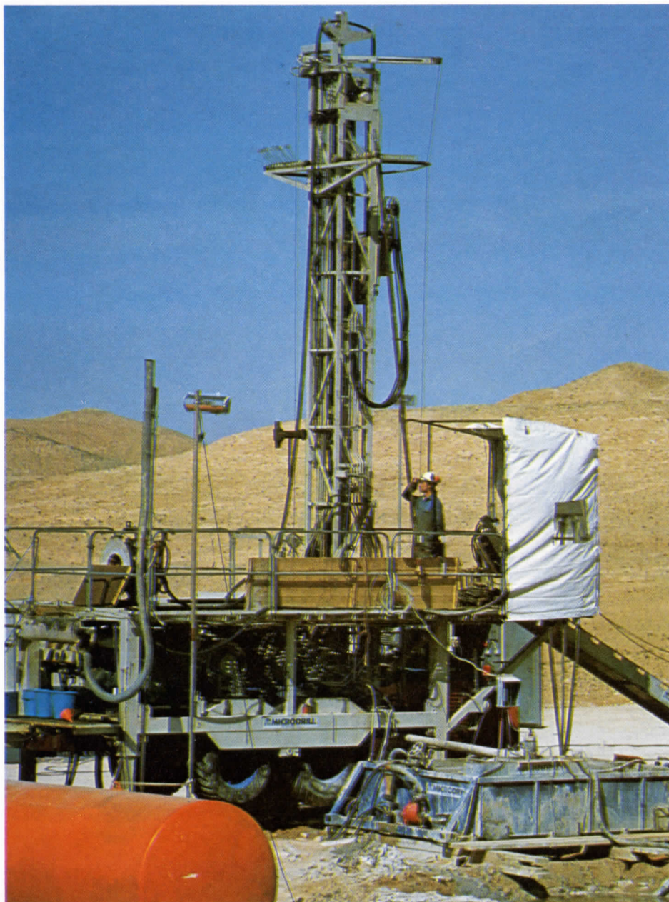
An advantage of the Microdrill technique is that it is less costly than conventional drilling, partly because it requires less personnel and the equipment is easily transportable.
